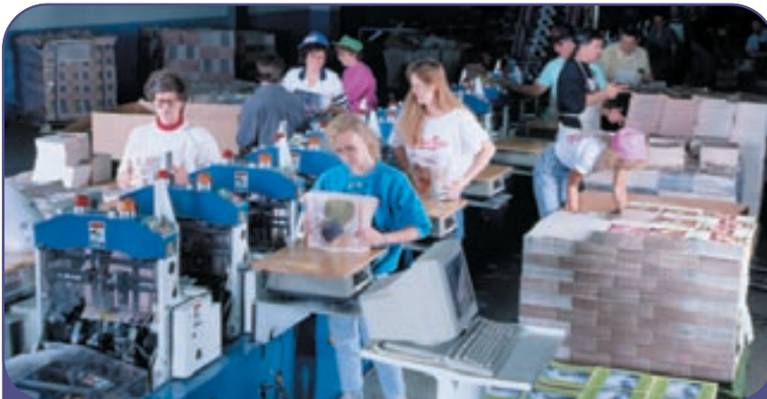
This newspaper operation utilizes many Model J-50 flat deck joggers to prepare inserts for newspaper insertion.
